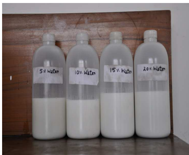
Fig. 5 Samples of water diesel emulsions by ratio of 5%, 10%, 15% and 20% of water in diesel
